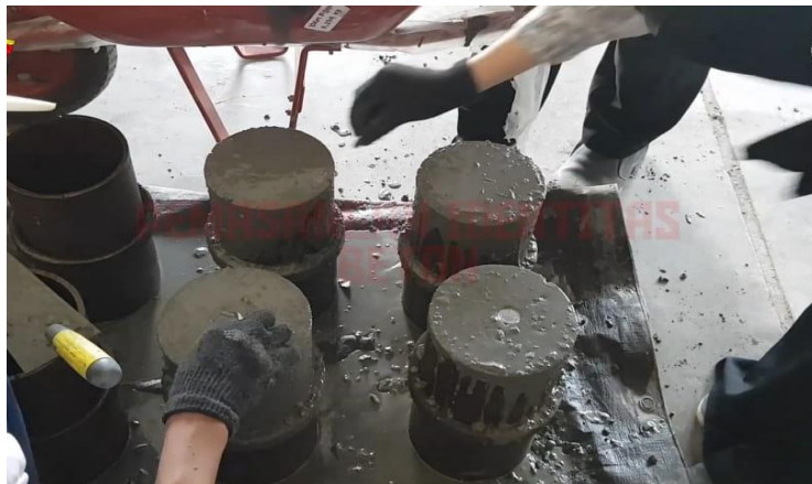
Figure 3. The casting concrete.
